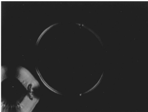
FIG. 2. Circular Sm-A filament grown from the I phase in the mixture of 8OCB and DODA (the molar concentration of 8OCB is 40%) observed at 36.4^\circ\text{C} . The picture is about 166 \mu\text{m} wide.
